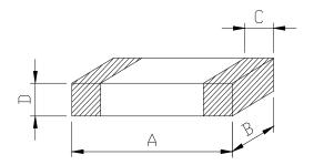
$\begin{array}{ccccccc} A & \vdots & 2.0 {\pm} 0.2 & m/m \\ B & \vdots & 1.25 {\pm} 0.2 & m/m \\ C & \vdots & 0.2 {\sim} 0.8 & m/m \\ D & \vdots & 1.25 {\pm} 0.2 & m/m \end{array}$
